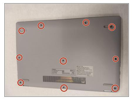
Remove the two rubber tabs near the front of the computer with a metal spudger and with PH0 Phillips head screwdriver, carefully remove all ten screws and place in a safe location.
