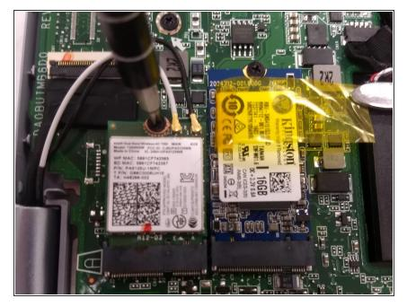
Carefully peel back the yellow tape by either folding it back or removing it entirely. Use the same PH0 Phillips head screwdriver to remove the single screw that connects the motherboard to the Wi-Fi PCB.
