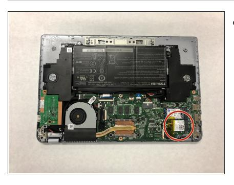
Ensure that there is no debris, dust, or any other foreign materials blocking the Wi-Fi PCB.
