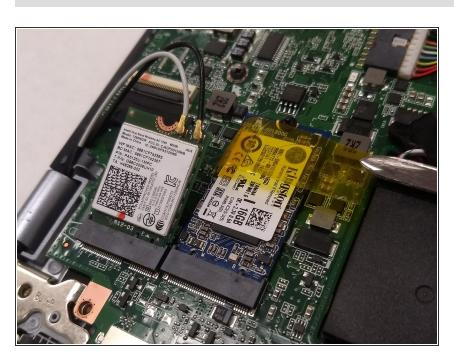
When the screw has been removed, the board will naturally spring up.
