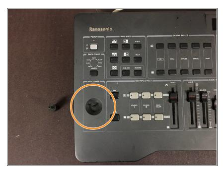
Unscrew the stick extension by turning it left. If you're running into resistance try holding the shaft of
