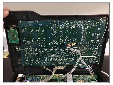
Shot of the solder-side of the topboard for reference on connector locations, cable routing, and component reference.
