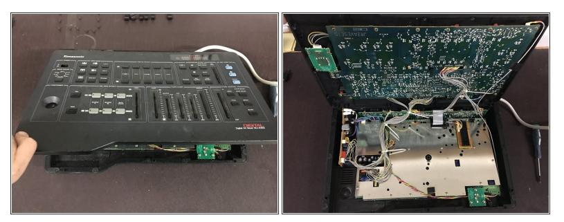
• Now the top-board should pivot up like a pizza-box allowing access to both the solder side of the top-board and the EMI Shielding for both the Primary Power Board and the Primary Control Board.
