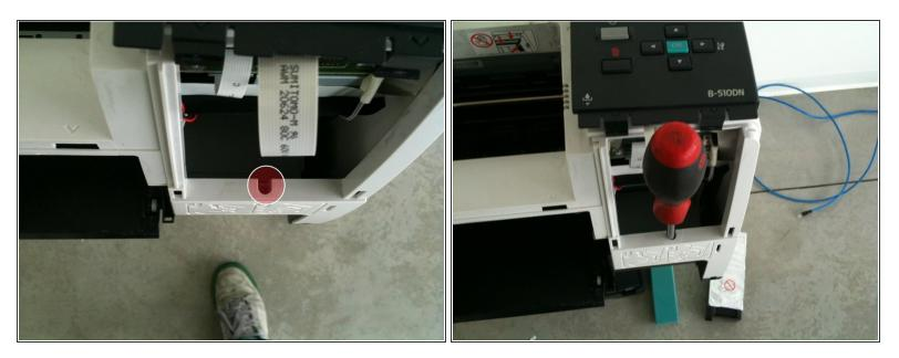
Remove the last back panel screw (hidden behind the LCD display)
