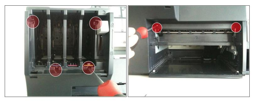
Remove the front panel screws
