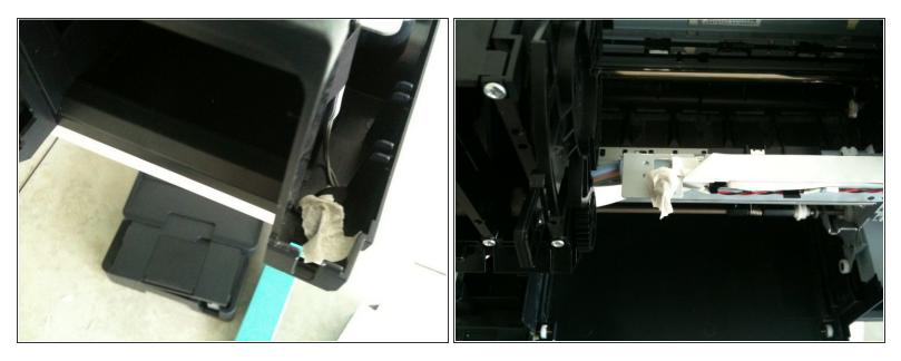
• If you want to test the printer you need to insert paper, and cover 2 switches with tape.
