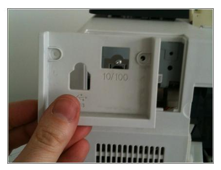
• Remove the back ethernet panel
