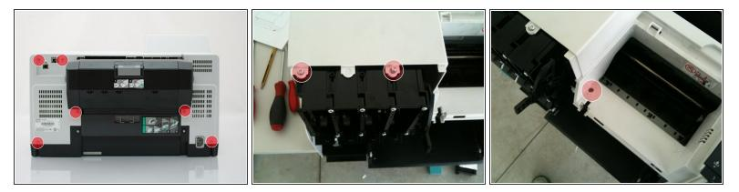
Remove the back panel screws
