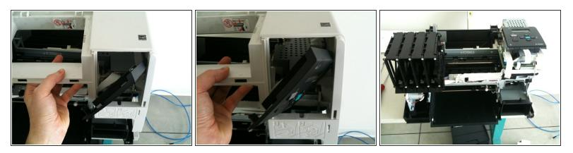
• Remove the main back panel, being careful not to damage the LCD display
