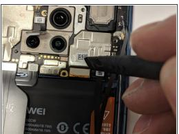
Standard ribbon cable attachments here need to be disengaged to get the PCB out. I prefer plastic spludgers. :)
