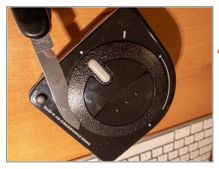
• Gently pry off the collar around the rotating piece. Do this on both sides.
