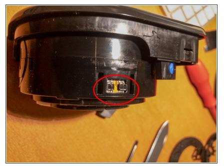
The housing contains the rotating barrel. On the barrel there are 2 (highlighted) reflective optical sensors used for identifying the position of the Colormunki's rotating part. Gently clean the sensors if you feel necessary. Use only a soft cloth, soak it in alcohol if needed.
