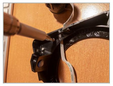
Remove the 2 small screws to release the plastic piece that holds the flat cable attached to the housing.
