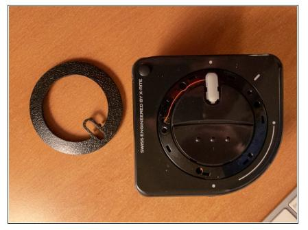
The collar is now removed. The small white plastic covering the LED light tends to fall off, be careful not to lose it.
