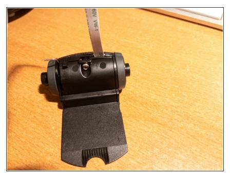
• Remove the small screw and gently pry open the small barrel.
