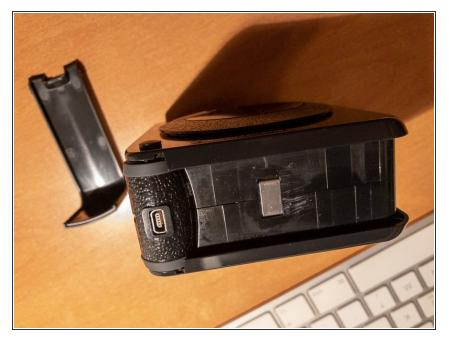
Once covers are removed you will see 4 metal clips connecting the 2 sides of the housing.
