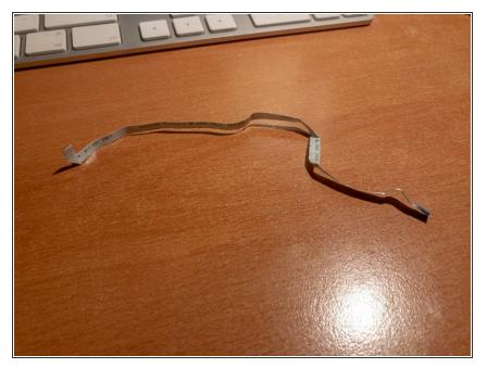
• Even if you have to replace it, retain the old cable in order to have a reference of where and how to bend the replacement for getting it back in place as intended.
