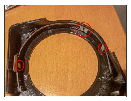
The light emitted by the sensors is bounced by the strips higlighted on the picture. Clean those if yo need to, or refurbish those by gluing on top reflective material (e.g. aluminium foil) while respecting the original shape and position of the strips.
