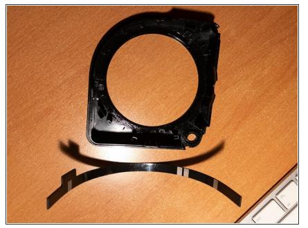
If you need to refurbish the reflecting strips, you can remove the plastic part holding the strips. This will allow you easier access to the strips.
