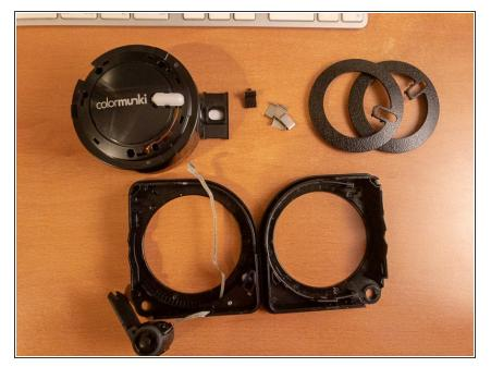
All parts dismantled except the flat cable from the USB port section.
