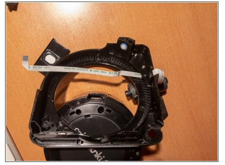
• You can read here the type of the flat cable. An equivalent replacement is part number 687708200002 from Wurth Electronics. It is also available via Conrad in Europe.
