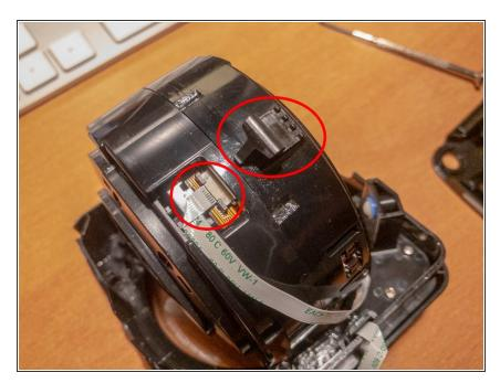
Remove the black plastic clip covering the flat cable's connection.
