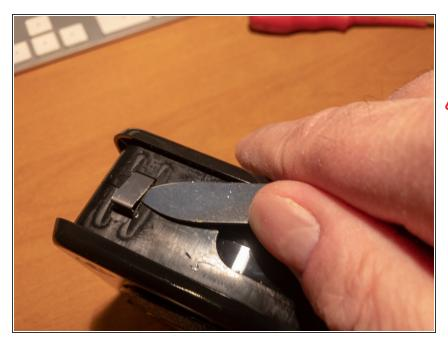
• Pry out the 4 clips that hold together the housing.
