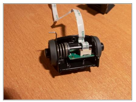
• As previously on the rotating barrel, distance gently the cable locking mechanism, i.e. the brown part from the white part. Once distanced you can easily remove the flat cable.
