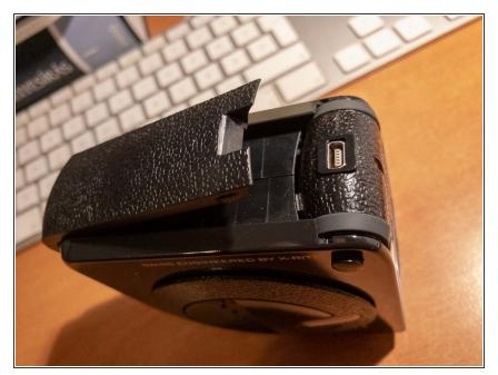
• Gently pry off the plastic covers. Start from the place indicated in the picture and go around. There are 3 cover pieces to be removed.
