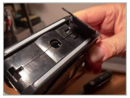
One of the clips is slightly hidden under the flipping part of the Colormunki.
