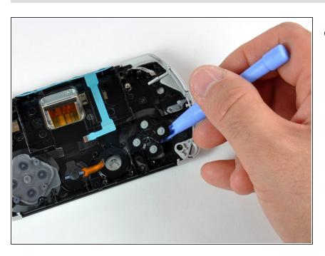
Use a plastic opening tool to take out the directional pad buttons.
