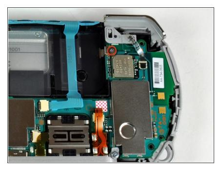
Remove the single Phillips screw securing the logic board to the inner case.
