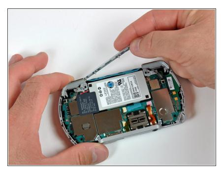
Pull the top cover upwards gently from its housing.
