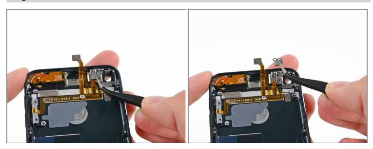
• Use <u>tweezers</u> to remove the small metal backing plate from the power switch section of the button ribbon cable.
