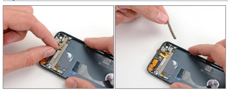
• Peel and remove the foam tape from the rear case of the iPod.
