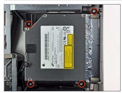
• Remove the four T10 Torx screws securing the optical drive to the outer case.
