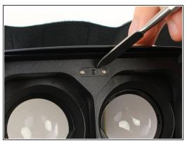
Use a metal spudger to remove the screw cover centered at the top.
