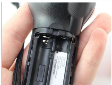
Remove the four 5mm Phillips #000 screws.
