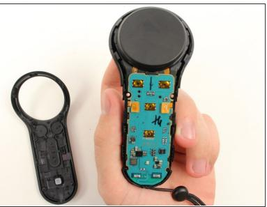
Pull apart the two halves of the controller to access the motherboard.
