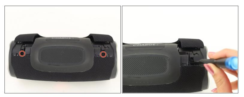
• Remove the two 8mm Phillips #0 screws from the other edge of the grille.
