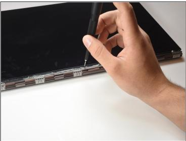
Remove the eight 3mm Phillips #000 screws that were below the metal cover to loosen the screen.
