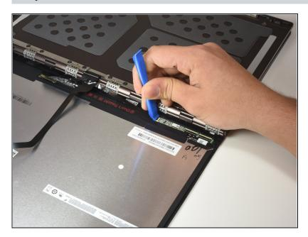
Flip up the black tab on the smallest connector at the bottom of the screen with the iFixit Opening Tool.
