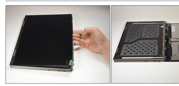
• Lift the screen with your hands and place the the screen face down, keeping the device in the same location.
