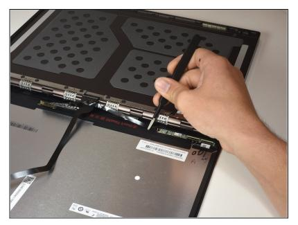
Use the iFixit Tweezers to remove the ribbon cable from the connector.
