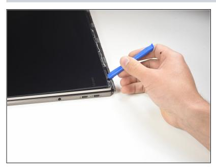
Pry up the screen with the iFixit Opening Tool.
