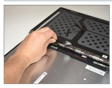
Remove the ribbon cable from the connector to detach the screen from the device.
