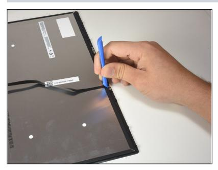
Flip up the black tab on the connector at the top of the screen with the iFixit Opening Tool.
