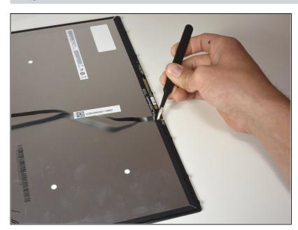
Use the iFixit Tweezers to remove the ribbon cable from the connector.
