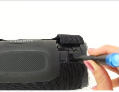
Remove the two 8mm Phillips #0 screws from the other edge of the grille.
