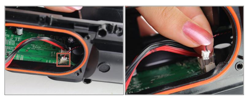
Remove the ground cable harness next to the speaker wire by gentling pulling it from the connector.
