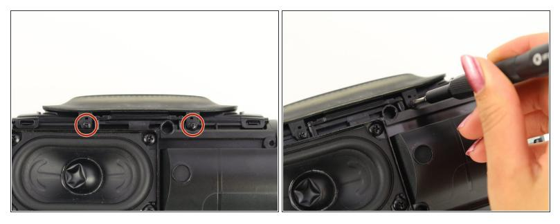
• Remove the two 6mm Phillips #0 screws on the front side of the port bay cover.
