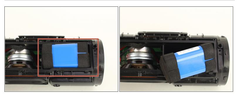
• Remove the battery from the battery socket by gently pulling on it.
