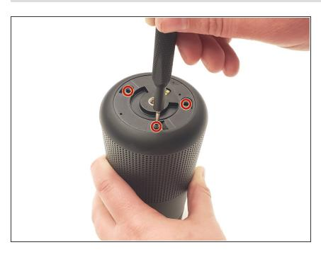
Use a T10 screwdriver to remove the three 10 mm screws from the bottom of the speaker.
