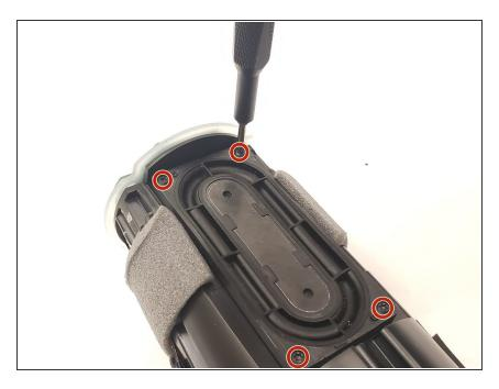
Remove the four 6 mm screws from the top part of the speaker body using a T10 screwdriver.
