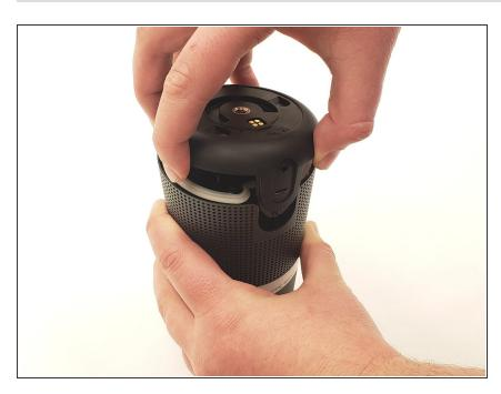
Unhook the ribbon conector that connects the bottom cover to the body, then remove the bottom part of the speaker.
