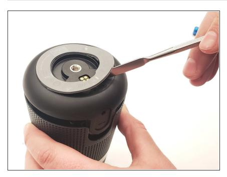
Use a plastic opening tool or metal spudger to remove the rubber mount from the bottom of the speaker.
