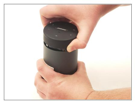
Use a TR9 screwdriver to remove the screws from the top of the speaker, and then remove the top part of the speaker along with the motherboard.
