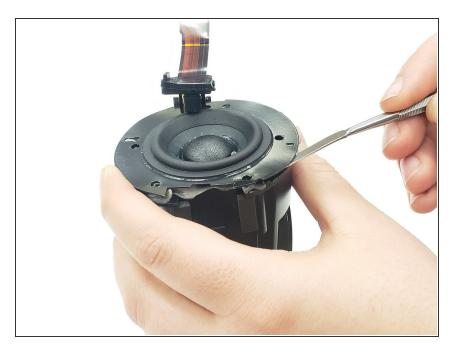
Use a spudger to pry apart the glued section between the speaker panel and the device.
