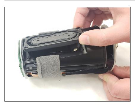
Remove the speakers from the device.
