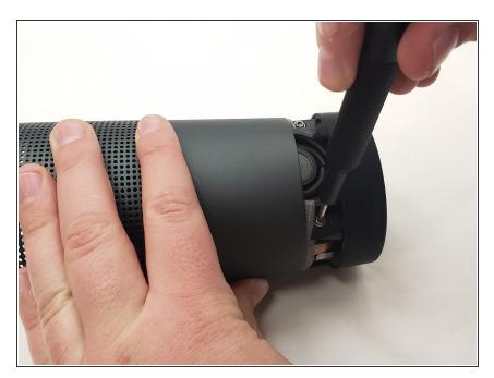
Use a T10 screwdriver to remove the four 6 mm screws around the 2 speakers, and remove the speaker units from the body.
