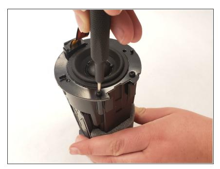
Remove the three 25.3mm screws from the bottom part of the speaker body with a T10 Torx screwdriver.
