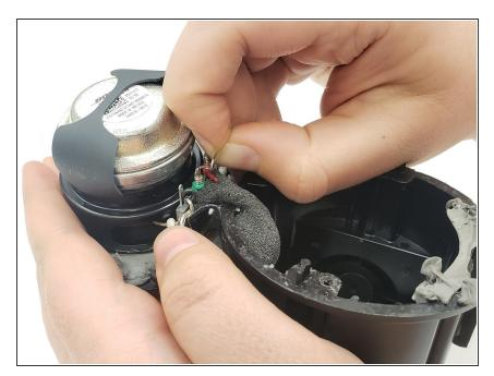
Open the speaker panel, then unwind the three wires from the speaker.
