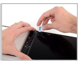
Insert the guitar pick into three more locations down the left side of the LCD and bend it over in each location, to slide the LCD over to the right side of the rear case.
