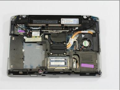
Remove the eight screws holding down the rear panel using a Phillips #0 Screwdriver. Carefully remove base cover by hand.
