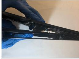
Pry the frame work of the laptop off using a plastic splunger.
