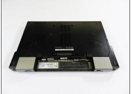
Pull the battery towards yourself as shown until completely removed from the computer.
