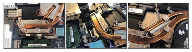
Loosen but do not remove the silver screws surrounding the heat sink using a PZ1 screwhead.
