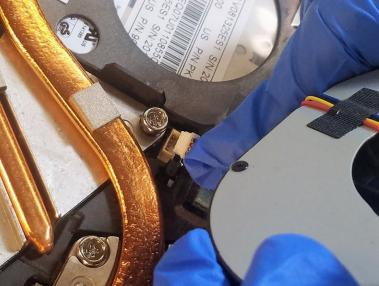
Locate the wire holding the fan in place and detach the clip.
