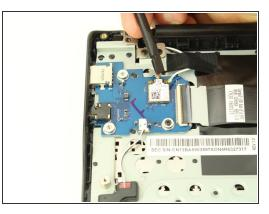
Pry the small coaxial cables upwards from the connecters on the wireless chip.
