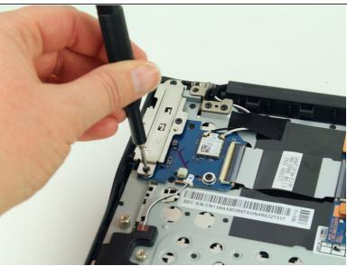
Before you begin the process of removing the daughterboard, you will need to remove the port case. Using a Phillips #00 screwdriver, remove the three 4.6mm screws.
