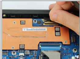
Disengage the gold connector joining the display and motherboard by flipping up the hinge with a spudger and gently disconnecting it with a spudger or your fingers.
