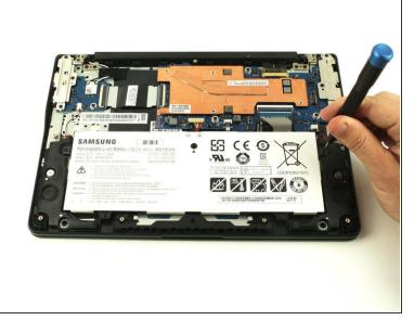
Locate the battery and remove the four 4.6mm screws at the corners which attach it to case using a Phillips #00 screwdriver.
