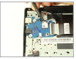
Next disconnect the small coaxial cables from the wireless chip on the daughterboard by prying upwards with a spudger.
