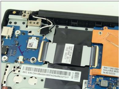
Flip up at least one side of the adhesive tape holding the coaxial cables in place. When the display is removed, the cables are coming with it!
