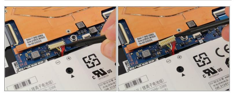
Use a spudger to gently pry the power cable cord upwards from the motherboard.
