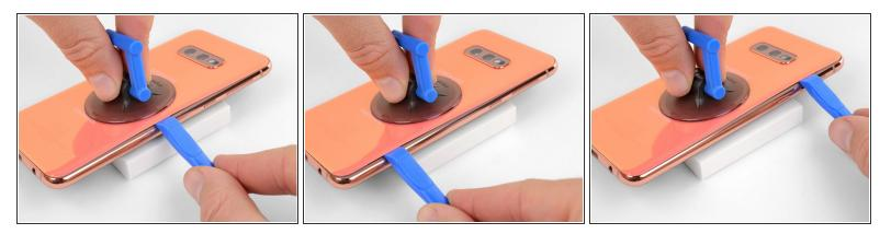
Slide the opening tool along the right edge of the phone to slice through the adhesive securing the back cover.
