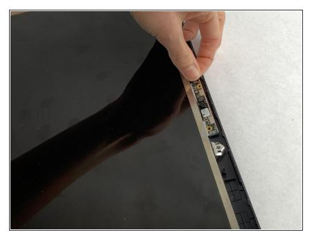
• Disconnect the webcam connector by gently pulling on the tabs using your hands or tweezers.
