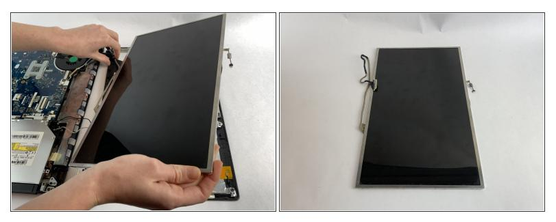
• Remove the screen completely.
