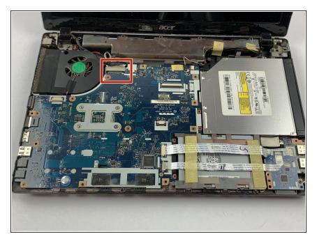
Locate the video cable connector keeping the screen connected to the motherboard.
