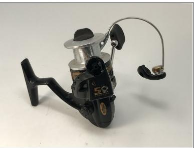
Place the new bail spring and pin back in the spring slot. Lightly push down on the spring to allow it to sit in its original position.
