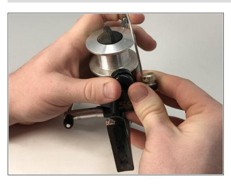
Line the bail back up with the reel, ensuring all holes align with each other. Lightly squeeze the bail and reel together to allow the two pieces to snap back together.
