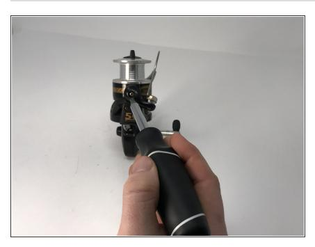
Remove the screw that holds the base of the bail arm to the reel with a Phillips #1 screwdriver.
