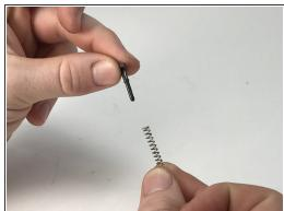
Replace the worn out bail spring by separating the pin from the spring. Then place the original pin inside of the new spring.
