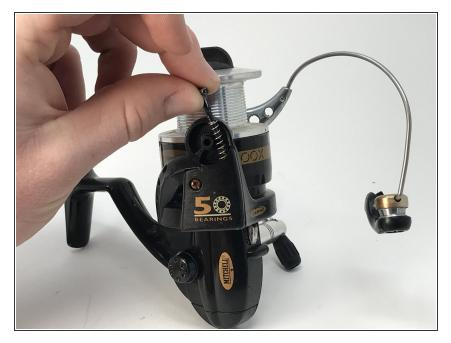
Remove the worn out bail spring by pushing down on the spring, then pulling outward away from the reel.
