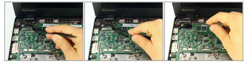
Use the flat end of the spudger to pop up the display cable connector from the motherboard.
