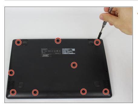
Use a Phillips #0 screwdriver to remove the nine 6mm screws from the larger back plate.
