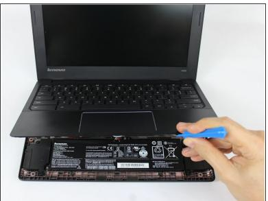
Turn your laptop back over, open it, and use the plastic opening tool on the recessed notch to gently pry each side and lift the keyboard plate up.
