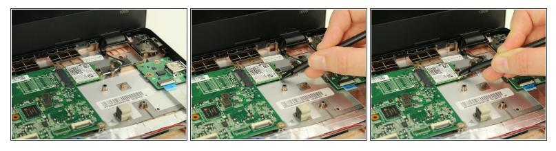
Pry up the coaxial antenna cables from the wifi card with the spudger.
