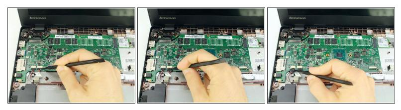
Use the spudger to coax the sliding speaker cables toward you, out of the motherboard attachments.
