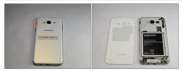
Remove the back of the device by pulling on the tab in the top left.
