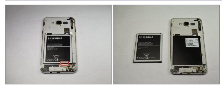
• Pull out the battery by pulling on the bottom left slit under the battery.
