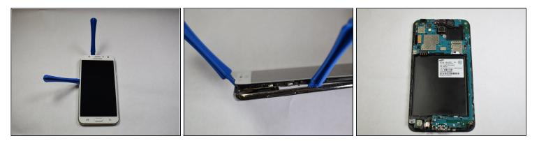
• Lift up the back of the device with the iFixit opening tool and disconnect it from the front.
