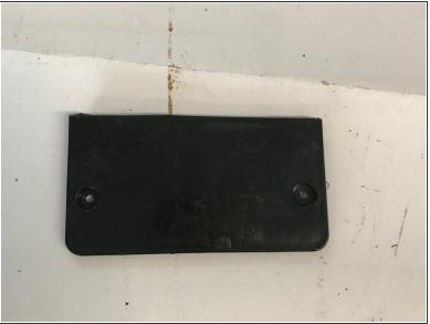
Now that the top is entirely dismantled, we can continue with the bottom. Turn the product around and remove all the screws from the bottom cover (this is where you'll need the Tamper Proof Spanner). The cover of the electronics will fall off automatically.
