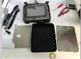
After that, we can disconnect the wires and take the heat shield of the upper heating plate. The
