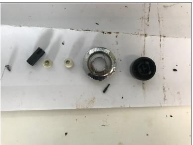
The last step is to take out the button and the covers of the neon indicator's. They are attached with snapfits, so can be pushed out.
