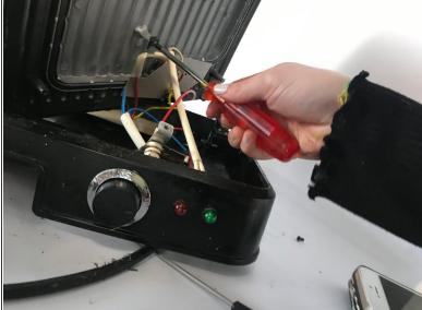
Next, the lower heating plate can be unscrewed. There are some wires attached that can be seen when lifting it up from the bottom cover.
