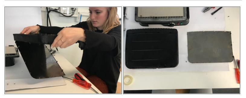
Now, take the top cover off. It should come off automatically, as the screws that held the side handles also held the top off the panini iron. Then, we can take of the metal top cover, by bending the pieces of iron that keep it together.
