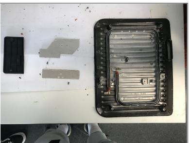
From the heating plate, we are now able to unscrew the heat shields.
