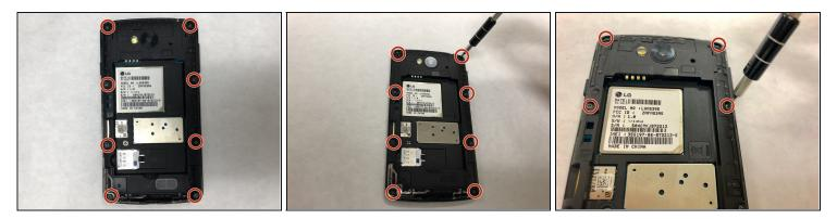
• Use the Phillips #000 Screwdriver to remove the eight 4mm screws.
