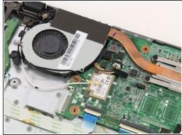
Use the spudger to gently disconnect the black and white coaxial antenna cables off of the WLAN card.
