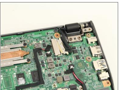
Use the spudger to disconnect the display connector from the motherboard.
