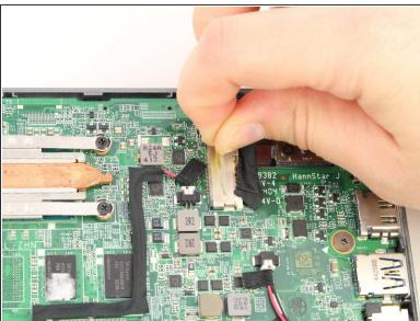
Using your fingers, pull the tape off of the display connector.
