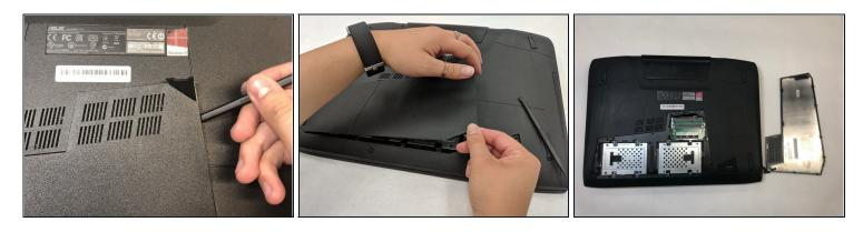
Use the standard spudger to remove the back center panel.
