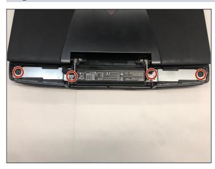
Use a Phillips 1 Screwdriver to remove the four 6.8 mm screws underneath the back panel.
