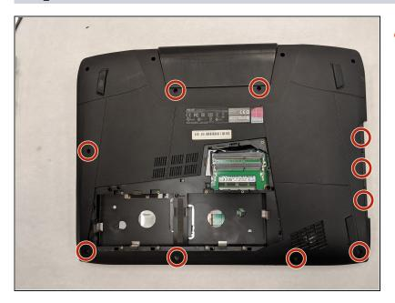
Use a Phillips 1 Screwdriver to remove the ten 5.2 mm screws holding the main panel in place.
