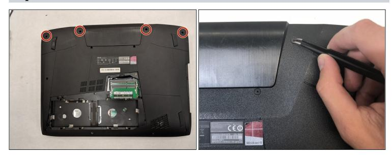
• Use a pair of <u>tweezers</u> to remove the top four rubber stoppers found on the bottom of the laptop.
