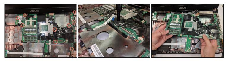
• Remove the screws holding in the motherboard using a Phillips 0 screwdriver.
