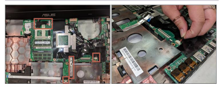
• Remove the ribbon cables connected to the motherboard.
