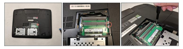
Use a Phillips 1 Screwdriver to remove the 5 mm screw that is located underneath the back panel.
