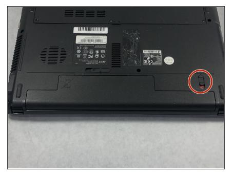
• Flip the lock latch to unlock battery.
