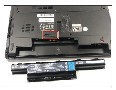
• Slide the middle latch and remove the battery.
