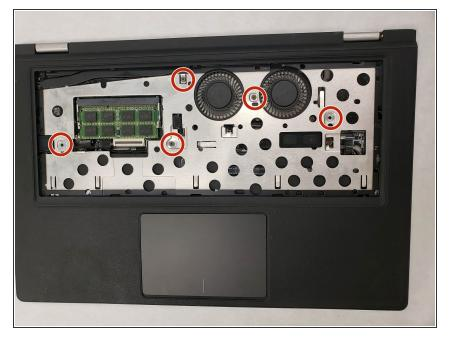
To remove the keyboard bezel, unscrew and remove the five screws using the Phillips #0 screwdriver.
