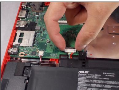
Using your thumb and index finger, pinch the multi-color cable and disconnect it from the motherboard.
