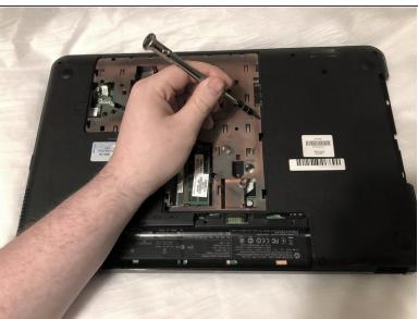
Using a Phillips #0 screwdriver, remove the optical drive anchor screw.
