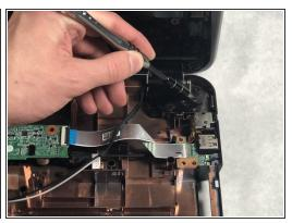
Using a Phillips #0 screwdriver, remove all six screws securing the display assembly hinges to the laptop.
