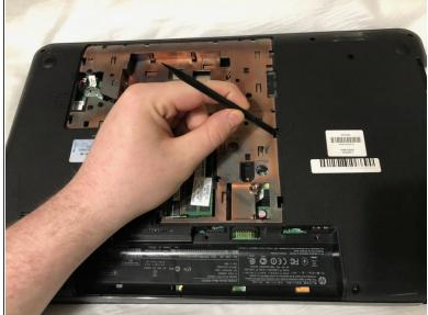
• Insert the flat end of a spudger into the optical drive release access hole.
