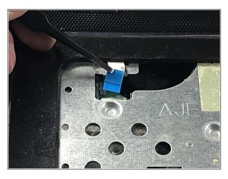
Using tweezers, pull the power ribbon cable free from the connector.
