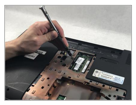
Using a Phillips #0 screwdriver, remove the Phillips M2.5×6.5 screw that secures the keyboard.
