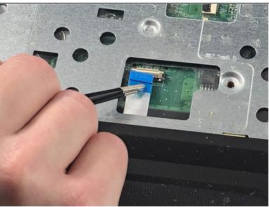
Using tweezers, pull the trackpad ribbon cable out from the connector on the motherboard.
