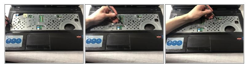
Remove the three Phillips M2.5 x 6.5 screws from the upper case assembly using a Phillips #0 screwdriver.
