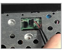
Using tweezers or a plastic opening tool, disconnect the speaker cable from the black connector located near the right side of the laptop.
