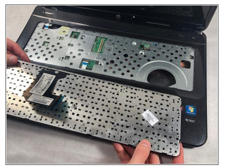
Remove the keyboard from the device.
