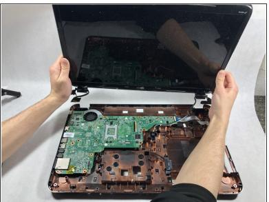
Lift up and remove the display assembly from the laptop.
