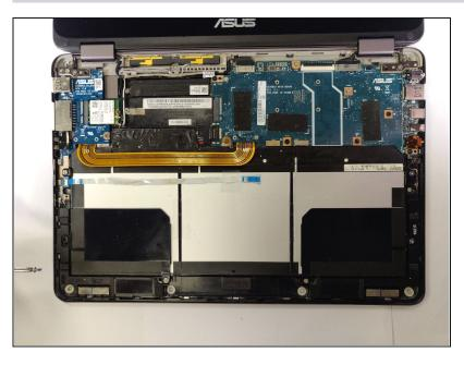
• Use the Phillips #1 screwdriver to remove all 5 mm screws.
