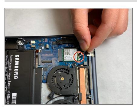
Gently pull off both cables attached to Wi-Fi card.
