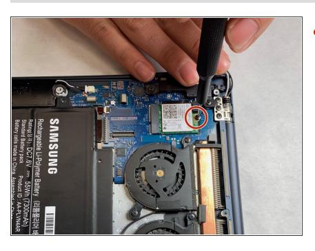
Unscrew the labeled screw using a Phillips #000 screwdriver.
