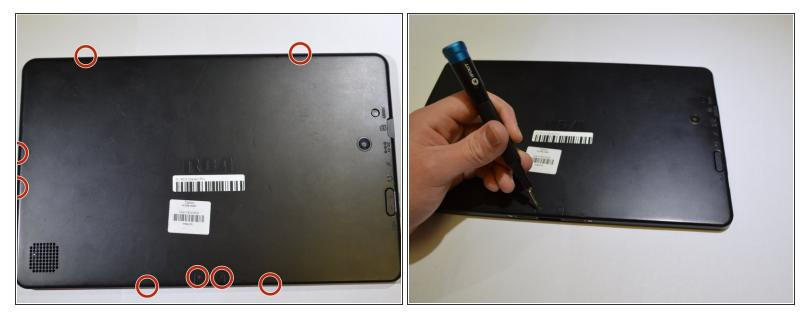
• Remove all the 8 mm Phillips head screws on the side and back of the device.
