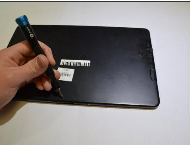
Remove all the 8 mm Phillips head screws on the side and back of the device.
