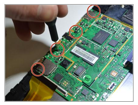
Use a Phillips head screwdriver to unscrew the 4 black screws that secure the motherboard to the device.
