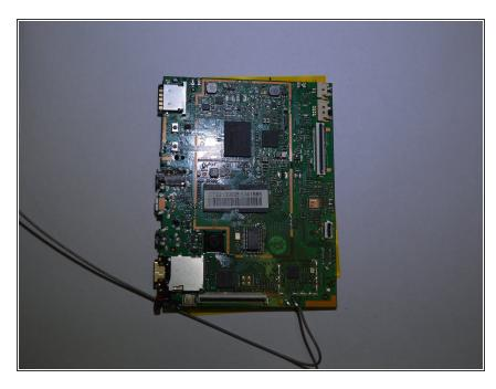
• Lift motherboard off the back of the tablet.
