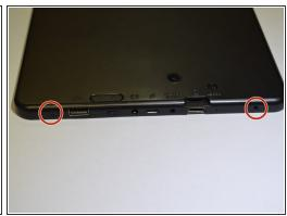
Use a Phillip's head screwdriver to unscrew the screws that secure the back cover in place. There
