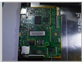
On the short edge of the motherboard, remove the yellow wire. To do this, lift up the clamp and pull out the wire.
