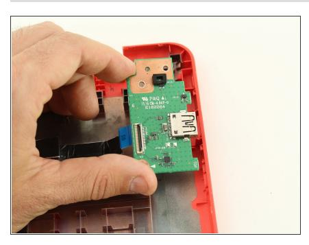
Remove the daughterboard by lifting it from the bottom case.
