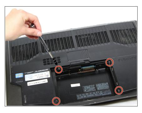
Unscrew the four 3mm screws with a J000 screwdriver.
