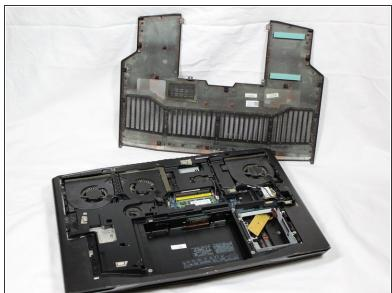
Use the iFixit opening tool to lift the bottom cover off.
