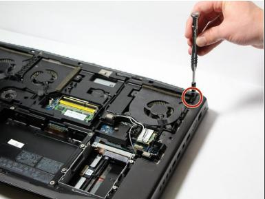
Remove the two 4mm screws with the J000 screwdriver.
