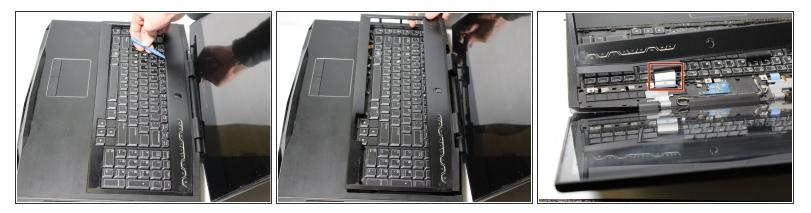
• The piece is now free from its fastenings to the base of the laptop, and can be lifted off.
