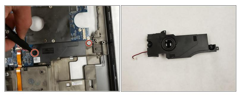
Remove the two screws on the speaker and lift the speaker out.
