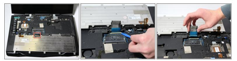
• Locate and remove the first connector cable.
