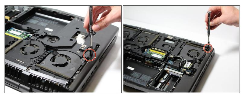
Remove the two 4mm screws with the J000 screwdriver.
