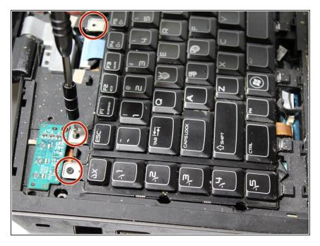
The keyboard's 3mm fastening screws are now exposed and can be removed with a J000 screwdriver.
