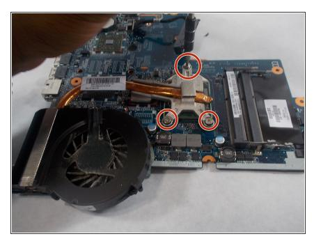
Use the Phillips #00 screwdriver to remove the three 2mm screws that connect the fan to the CPU.
