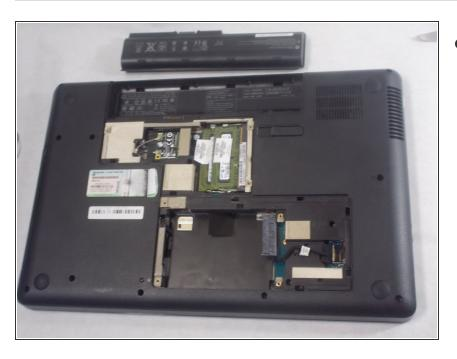
Remove the battery, RAM, and hard drive.
