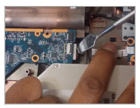
Unplug the wires connected to the motherboard with a spudger.
