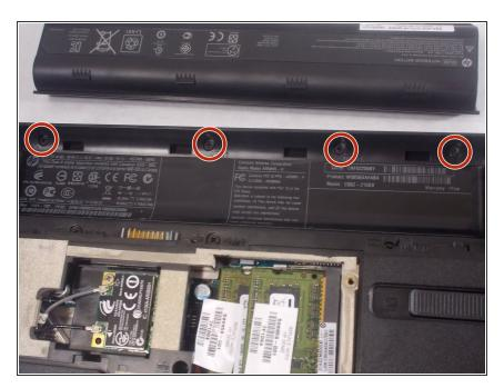
Remove four 1.2mm Phillips #00 screws under the battery.
