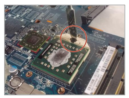
Use the metal spudger to twist the lock tab on the component.
