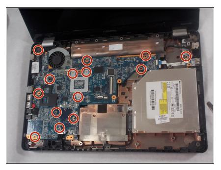
Remove all the 1.2mm Phillips #00 screws from the motherboard and in the top corner that secures the fan.
