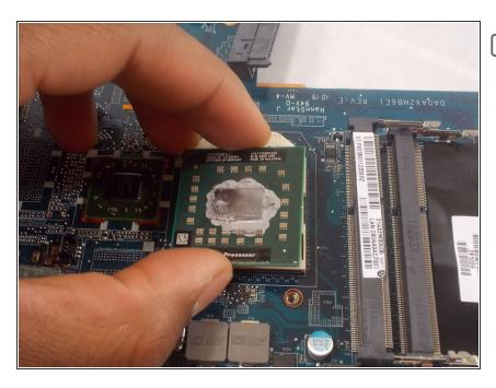
Remove current CPU and replace with new component.
