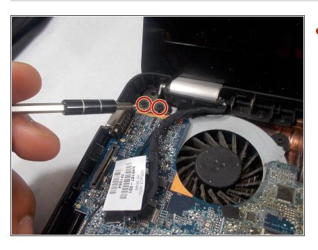
Remove the two 3mm Phillips #00 screws beside the fan.
