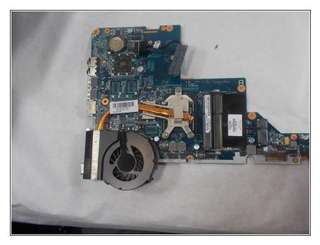
When the motherboard is removed, flip it over, and you will have a view just like in the picture.
