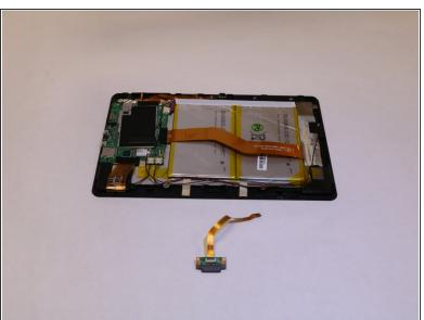
Remove the connector by lifting it upward.
