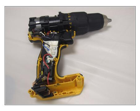
Lift drill mechanism from the drill assembly.
