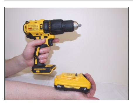
Pull the battery in a horizontal direction away from the drill.
