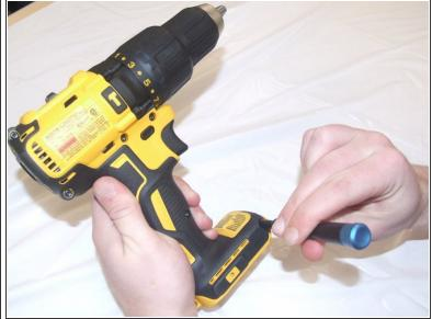
Remove the eight 16 mm, Torx Security #15 screws.
