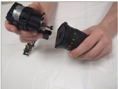
Slightly twist and pull motor away from the clutch.
