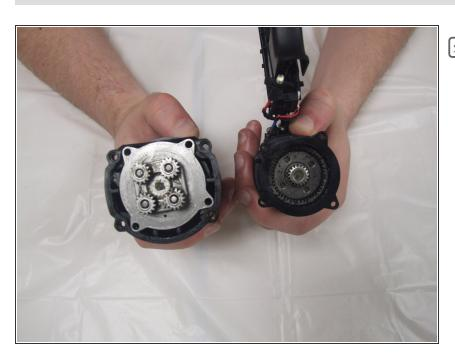
When installing the replacement motor into the clutch make sure you correctly align the gears in order to assure that the motor is properly fitted to the clutch.
