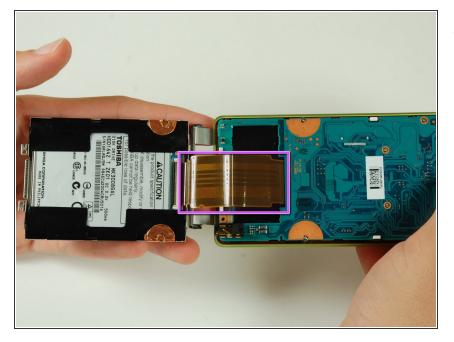
• Flip the hard drive over the top to expose the ribbon cable.
