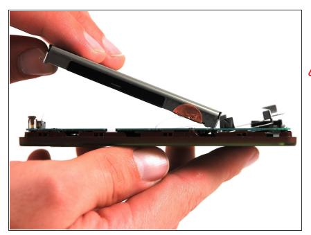
• Carefully tilt the hard drive up from the logic board.
