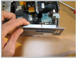
To remove the side panel of the case- gently pry around the corners until removed
