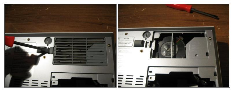
• Then simply pry up on the intake air door and remove
