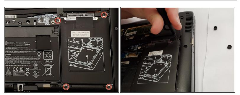
• Use a Phillips #0 screwdriver to unscrew the four 2 mm screws that secure the hard drive.
