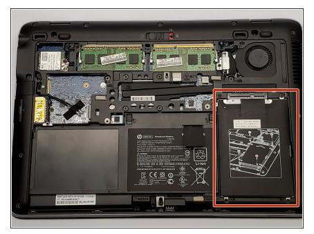
The hard drive is found on the bottom right under the back panel.
