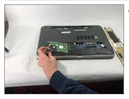
Grabbing from the left of the hard drive, slide the part to the left and pull up, lifting it away from the machine.
