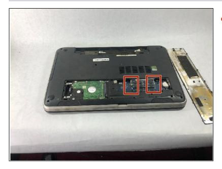
Using your fingers, separate the metal tabs located on the left and right of each stick of RAM by pulling them apart from each other.
